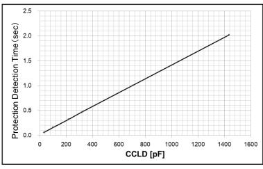
CLD Terminal Capacitance (pF) (VCC=12V,Ta=25deg)
