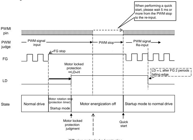
※During motor locked protection, the shift to STBY mode does not occur even after PWM stop input.
