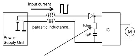
The current peak is reduces according to adding in series with bypass capacitance.
