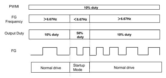
For example, when the rotational speed of the motor drive with input PWM = 10% and output drive duty = 10% in SEL = Open setting becomes 6.67Hz or less as FG frequency, Since the shift to the startup mode, the output duty becomes 50%, and as a result, the rotation speed in this section rises momentarily and shift to the normal drive mode, the output drive duty becomes 10%.
