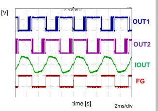
condition :  $V_{CC} = 24V,PWMI=100\%duty$  $C_{VCC} = 1\mu F,$
