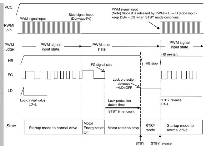
Since STBY mode is released by PWMI =  $L \rightarrow H$  (edge input), keep Duty = 0% when STBY mode continues. If the PWMIN pin is open (HiZ) in STBY mode, the STBY mode is released.
