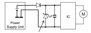
Add the zener diode in parallel with bypass capacitance
